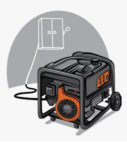
A transfer or throw switch is an essential mechanism that safely shuts off power to the electrical grid before backup power is used. This switch is sometimes referred to as a double-throw switch, as it controls two separate circuits.
